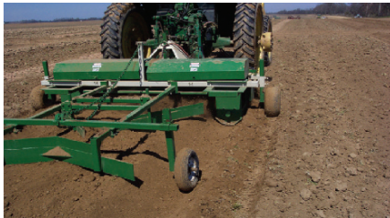
Plate 15 Sweetpotato bed covering machine, covering seed potatoes (Courtesy of Tara Smith, Louisiana State University Agricultural Center) (See also Plate 14.2 on page 300)
