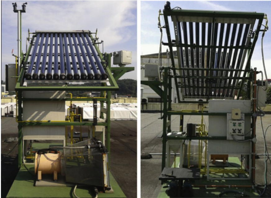
Fig. 4 Evacuated solar collector experimental setup used in [82]
