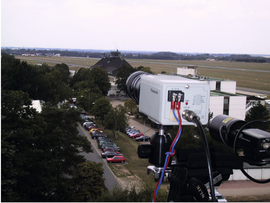
Fig. 4 Initial tests (2003) of video-based far view reconstruction with standard video technology. Camera position on DLR telemetry antenna tower, ca. 25 m above ground. Camera aiming at Braunschweig airport tower on the dark roof top. White building to the right is location of initial experimental videopanorama camera system (chapter “Remote Tower Experimental System with Augmented Vision Videopanorama”). Runway visible above the camera, extending in west direction
