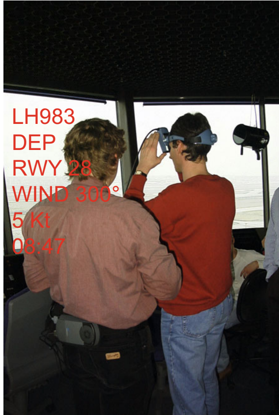
Fig. 2 Demonstration of a laser retinal scanning display, tested by operational controllers at Frankfurt tower (2/2003). Inset: superimposed text depicts augmented vision information displayed by HMD via direct image projection onto the retina by means of a laser scanner. Wearable HMD-computing device at the back of DLR team member Markus Schmidt
