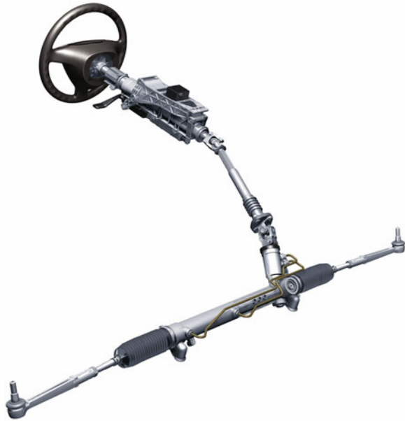
Fig. 1.1 Components of a steering assembly ( Porsche 997 )
