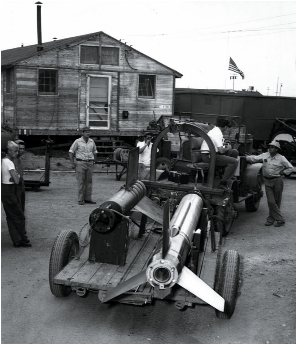
The WAC Corporal was America's first high-altitude 'sounding' rocket. It had a short duration solid propellant booster (visible on the left) and liquid propellant main stage. It was first launched at the White Sands Proving Grounds in New Mexico in 1945. (White Sands Missile Range)
