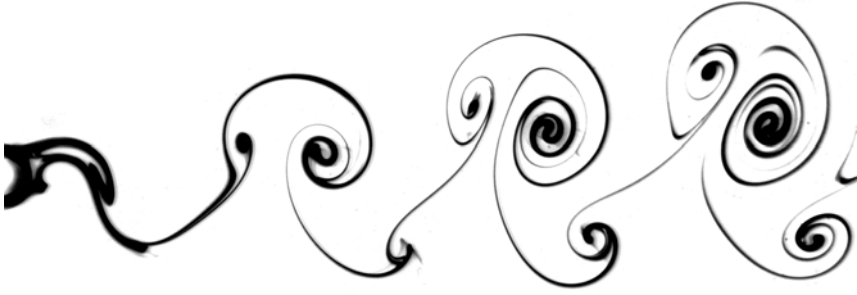
Fig. 4. “Exotic” vortex street wake behind an oscillating cylinder (courtesy of C.H.K. Williamson).
