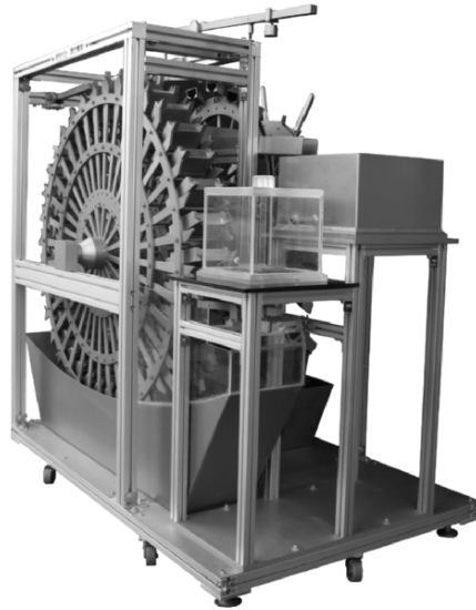
Figure 1.9 One possible reconstruction design of Su Song's water wheel steelyard-clepsydra device
