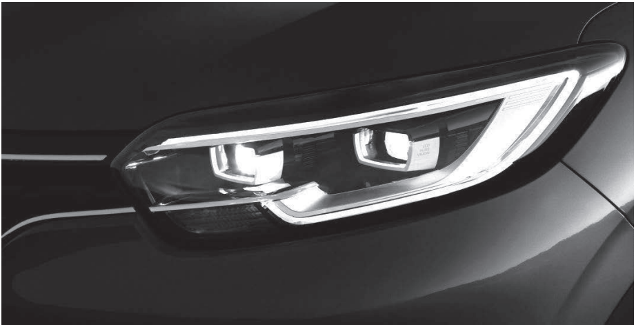
Figure 3: RENAULT KADJAR full LED headlamp with light signature
