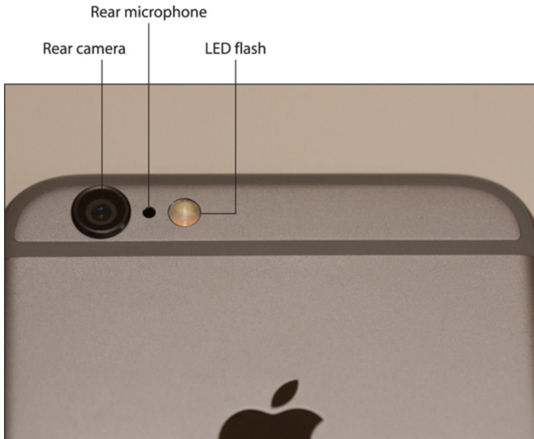
1.7 The back of the iPhone is where you'll find the rear camera and its LED flash.
