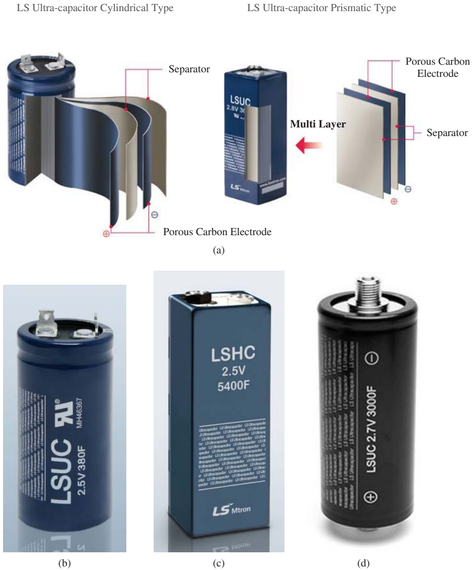
Figure 1.7 LS Mtron ultra-capacitors. Copyright LS Mtron, with permission
