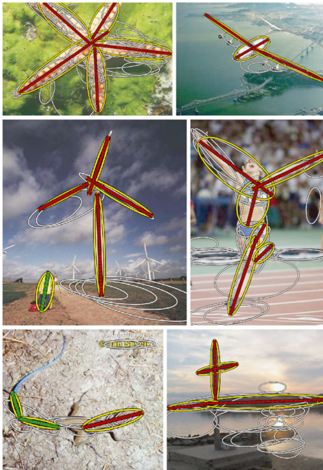
Fig. 1.5 Detected medial parts and their clusters. Parts with the same color axis have been grouped together (through high attachment affinities) and are hypothesized to belong to the same object. (Figure reproduced with kind permission from Springer Science+Business Media: Proceedings, 4th Mexican Conference on Pattern Recognition (MCPR) , Perceptual Grouping using Superpixels, 2012, S. Dickinson, A. Levinshtein, and C. Sminchisescu, p. 18, Fig. 3)
