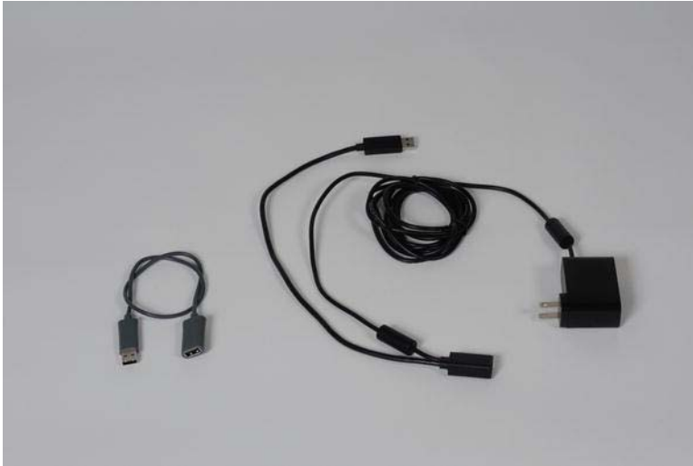
Figure 1-4. Kinect USB extender on the left for newer Xbox systems, and the Kinect power adapter on the right.
