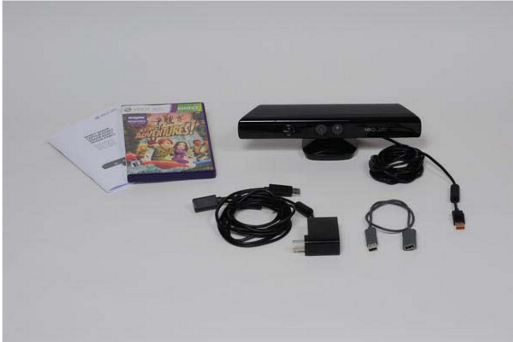
Figure 1-5. Contents of standalone Kinect sensor box: Manual, Kinect Adventures! game disc, the Kinect itself, AC adapter, and special USB extender.
