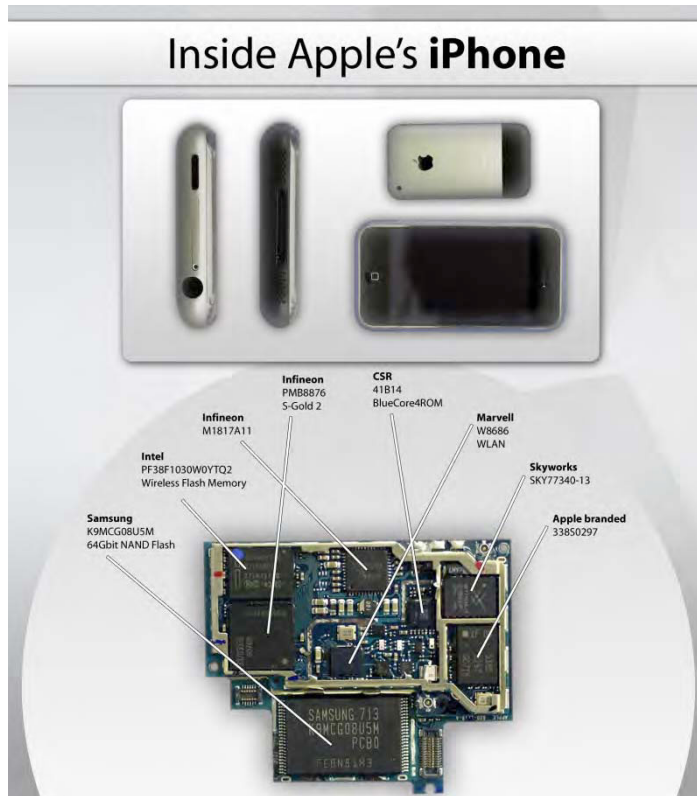
Figure 1–9. The internals of the Apple iPhone 2G (courtesy of Semiconductor Insights)
