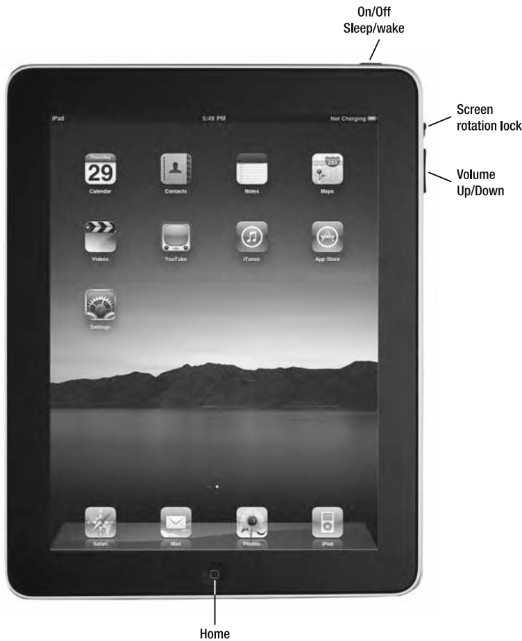
Figure 1-3. Feature breakdown displaying the buttons on the sides and front of the iPad. The dock connector port is on the bottom of the iPad near the Home button.
