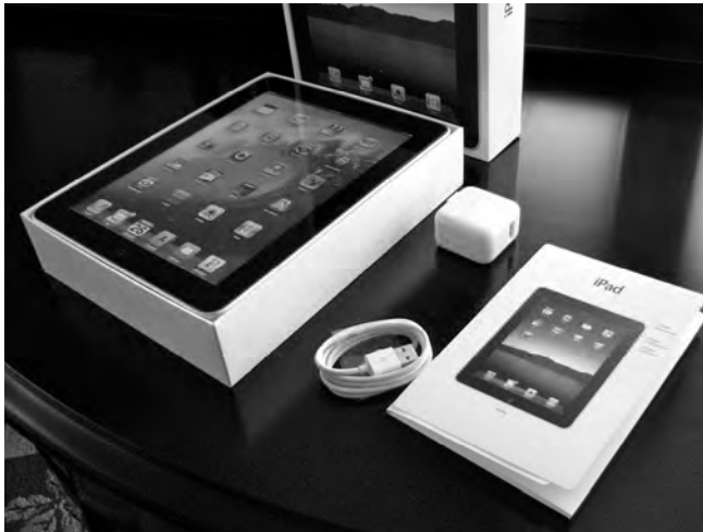
Figure 1-2. There's not much inside the iPad box: the iPad, a Dock Connector to USB cable, a 10-watt AC adapter, and some simple documentation.
