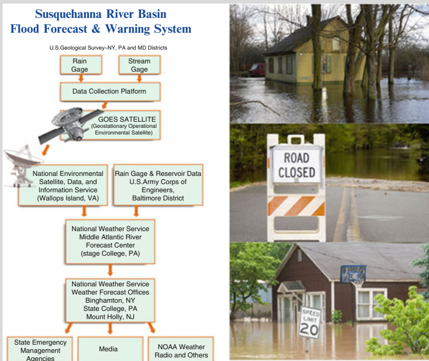
Fig. 1.4 Schematic of the Susquehanna Flood Forecast and Warning System (SRBC 2011) and images from the system website http://www.susquehanna flood forecasting.org/
