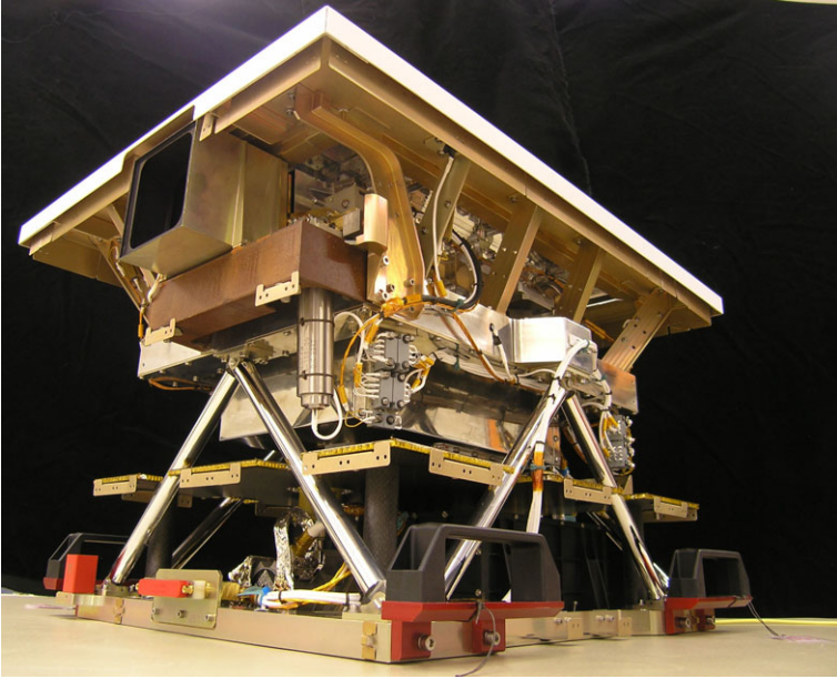
Fig. 7 The visible and infrared (VIR) spectrometer provided by the Italian Space Agency (ASI) and the Italian National Institute for Astrophysics (INAF). (Credit: Selex Galileo, INAF, and ASI)
