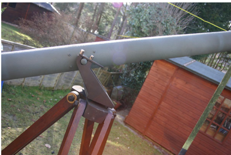
Fig. 1.2 The alt-azimuth head of the Dollond Student's refractor
