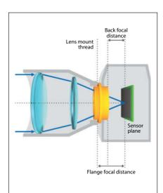
Differences in flange depth mean that the thickness of the adapter determines the focusing accuracy of your combined camera/lens unit
