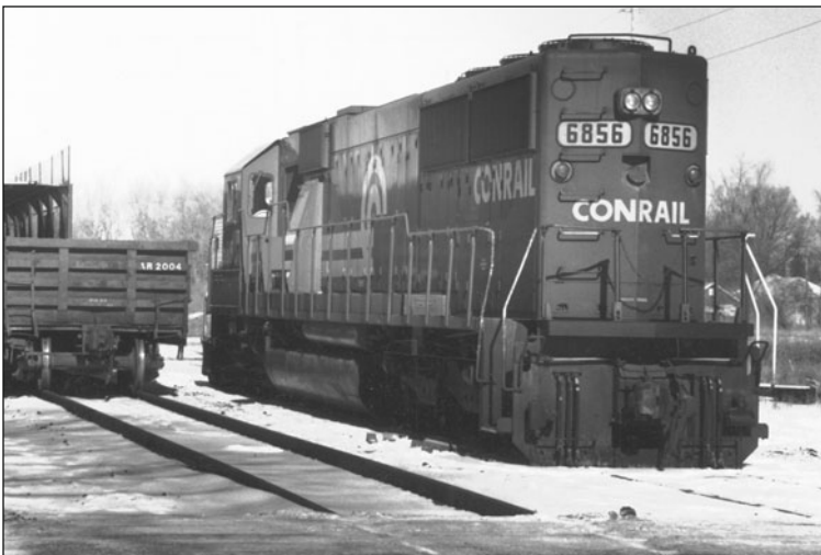
Fig. 1.12. A combination of snow and extremely cold temperatures left icing on the rails leading to the derailment of the leading wheels of this Conrail SD60 engine sitting in a rail yard in western Pennsylvania.
