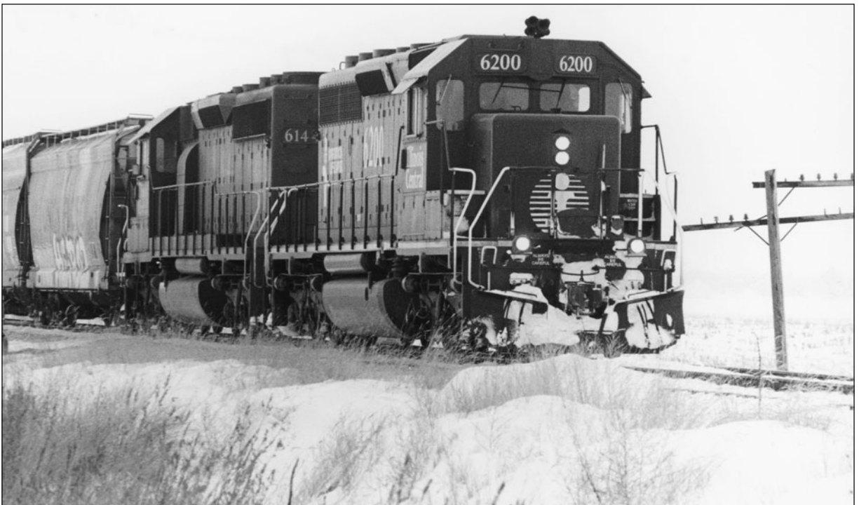
Fig. 1.7. Deep snow impedes train movement. Here an IC grain train struggles through a 15-inch snowfall with heavy drifts on the rail line in northern Illinois.
