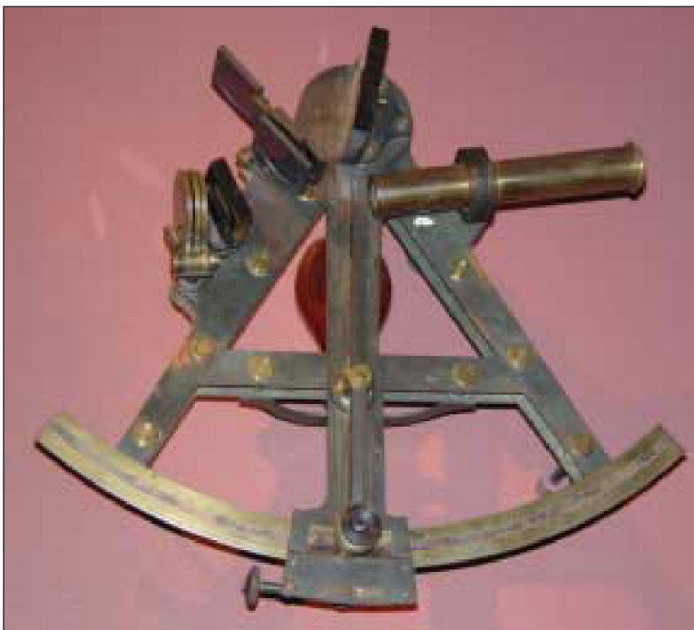
A sextant used for astronomical observations to determine latitude for navigation. Photograph taken at Jefferson National Expansion Memorial. (See April 5, 1806.)
