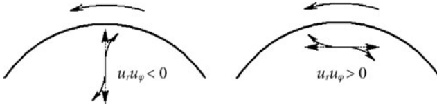
Figure 1.12 Illustration of angular momentum transport by rotating turbulence. The direction of rotation is shown at the top. See text.
