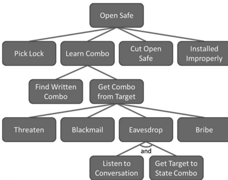
Figure 1-3. Bruce Schneier introduced attack trees to help analyze the sequence of events involved in a successful attack, starting from the outcome and working backward. 2
