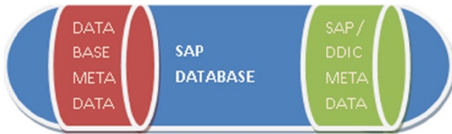
Figure 2-3. The two distinct sets of metadata in the SAP database: Database metadata and DDIC metadata
