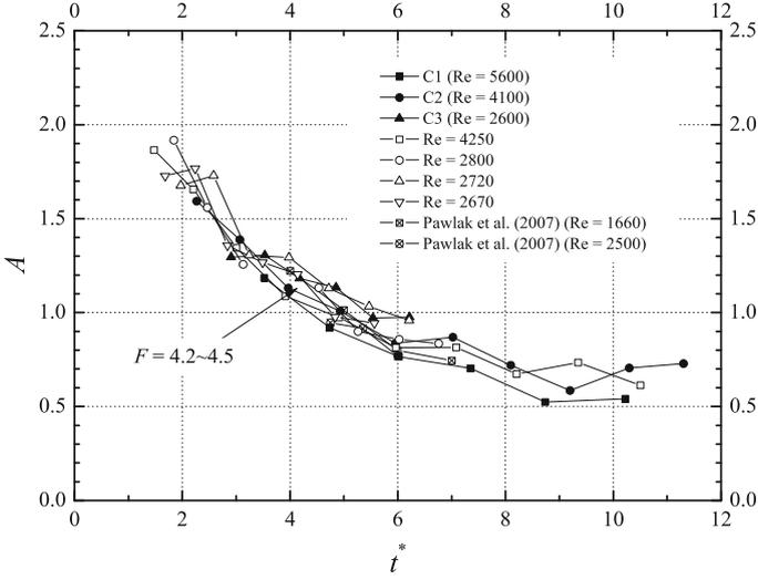
**Fig. 6** The variation of the instability parameter  $A$  against the formation time  $t^*$ . The data of Pawlak et al. [45] are also included for comparison (graph reproduced from Gao and Yu [15])
