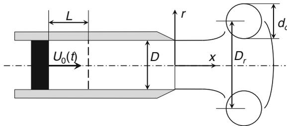
**Fig. 1** Illustration of a starting jet generated by the piston-cylinder apparatus and the formation of a leading vortex ring
