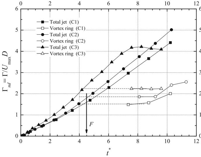
**Fig. 4** The circulation method for determining the formation number  $F$  (reproduced from Gao and Yu [15])
