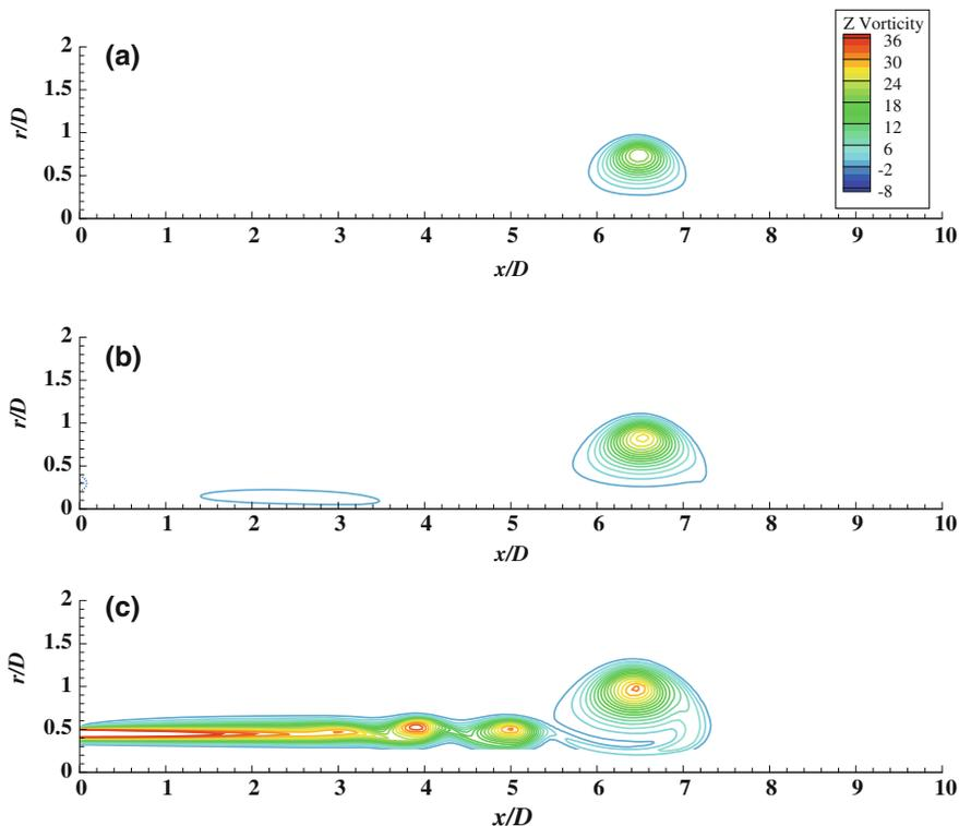
**Fig. 2** Vorticity contours of flow field for the starting jets with maximum stroke ratio: **a**  $L_{max}/D = 2$ , **b**  $L_{max}/D = 4$ , and **c**  $L_{max}/D = +\infty$ , when vortex rings translate at downstream location  $x/D \approx 6.5$ . The minimum absolute vorticity value shown is  $2 \text{ s}^{-1}$
