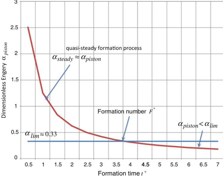
**Fig. 5** Explanation of the vortex ring pinch-off process based on the Kelvin-Benjamin variational principle
