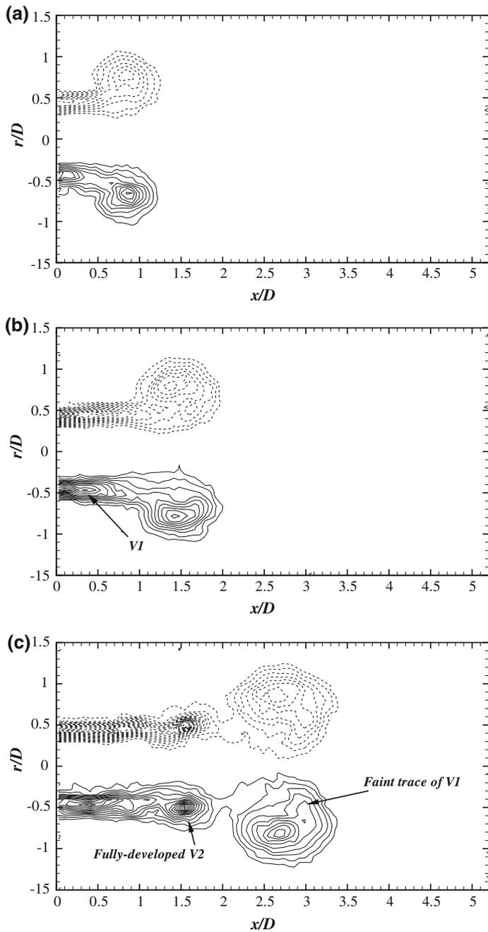
**Fig. 3** The evolution of vorticity contours of a starting jet at: **a**  $t^* = 3.1$ , **b**  $t^* = 4.9$ , **c**  $t^* = 8.1$ . The formation number for this case is  $F = 4.5 \pm 0.1$ .  $V1$  and  $V2$  indicate the first and second trailing vortices, respectively. Graphs are reproduced from Gao and Yu [15]
