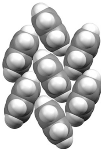
Fig. 1.6 Crystal structure and intra-layer transfer integrals of thin-film pentacene [5]
