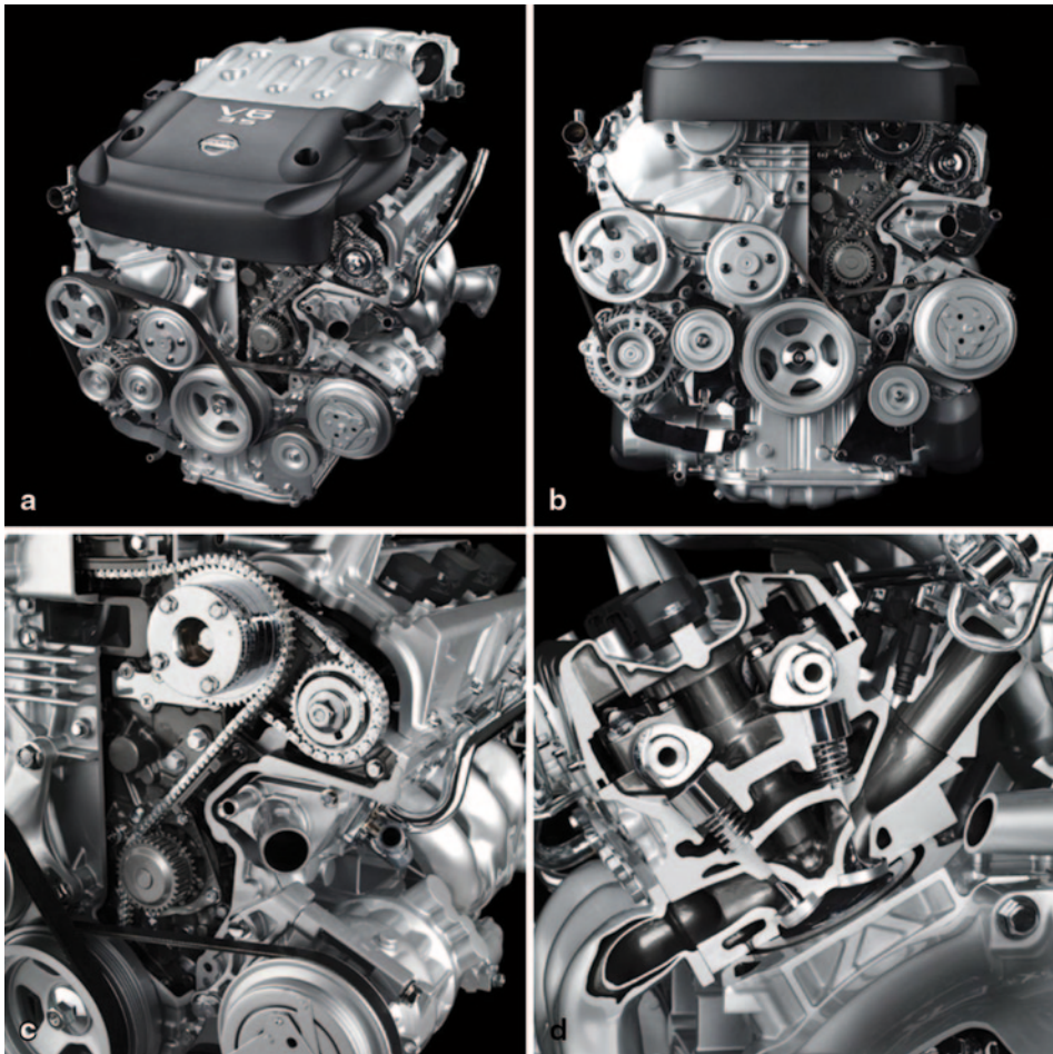
Fig. 1.7 a Double-overhead cam V6 engine, with cut-away showing cam drive chain (Courtesy of Nissan Motor Company). b Front view of engine shown in Fig. 1.7a. Serpentine belt accessory drives and cam drive cut-away are shown (Courtesy of Nissan Motor Company). c Details of cam drive, showing variable timing device for the intake camshaft. Engine is again that of Fig. 1.7a (Courtesy of Nissan Motor Company). d Cylinder head, intake and exhaust manifold cut-away for engine of Fig. 1.7a (Courtesy of Nissan Motor Company)
