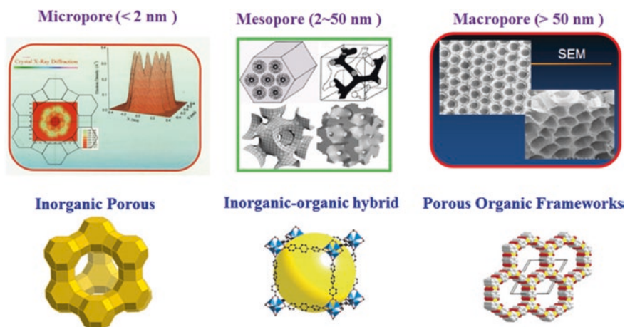
Fig. 1.2 Porous materials could be classified according to their pore size and their components
