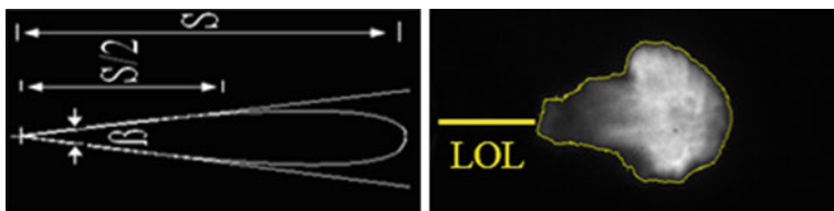
Fig. 4 Definition of spray characteristics ( S = Penetration Length, LOL = flame lift-off, \beta = spray angle)
