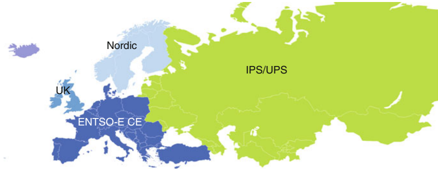
Fig. 1.2 Geographical representation of synchronous areas in Europe (ENTSO-E and IPS/UPS) (Map: © Lutum+Tappert)
