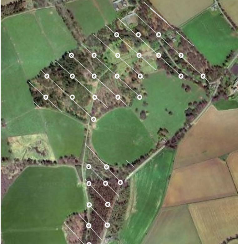
Fig. 2.1 The survey design for the Montrave study. The surveyed woodland and parkland totalled about 33 ha in two blocks, surrounded by grazing and crops. For the point transect surveys, a systematic grid of 32 points (indicated by circles ) was placed over the study area, with 100 m separation between neighbouring points. Each point was visited twice. For the line transect survey, there were 19 lines (11 in one block and eight in the other), with about 70 m separating successive lines. Each line was surveyed twice
