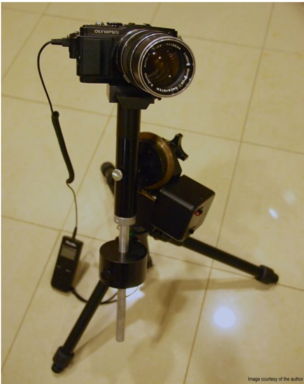
Fig. 1.3 Pocono II GEM on miniature tripod with OM series 135 mm f/3.5 lens and intervalometer
