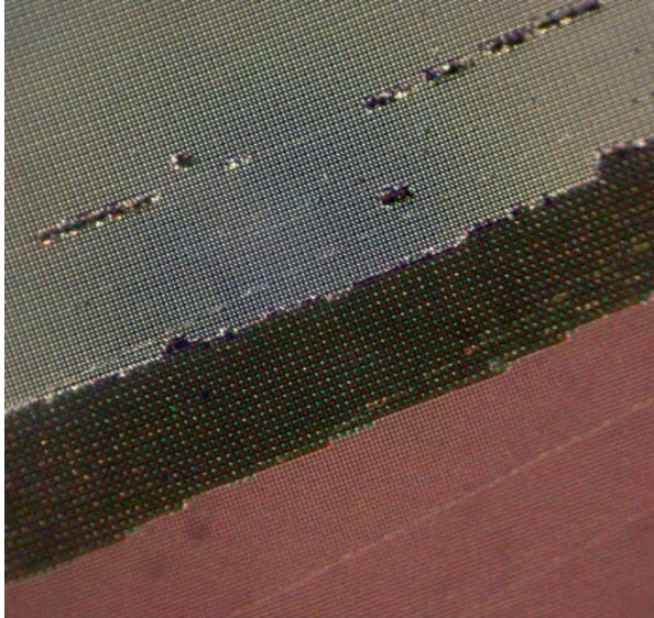
Fig. 1.8 View of sensor surface at 100× magnification. From top to bottom : naked pixels, Bayer layer, microlens layer
