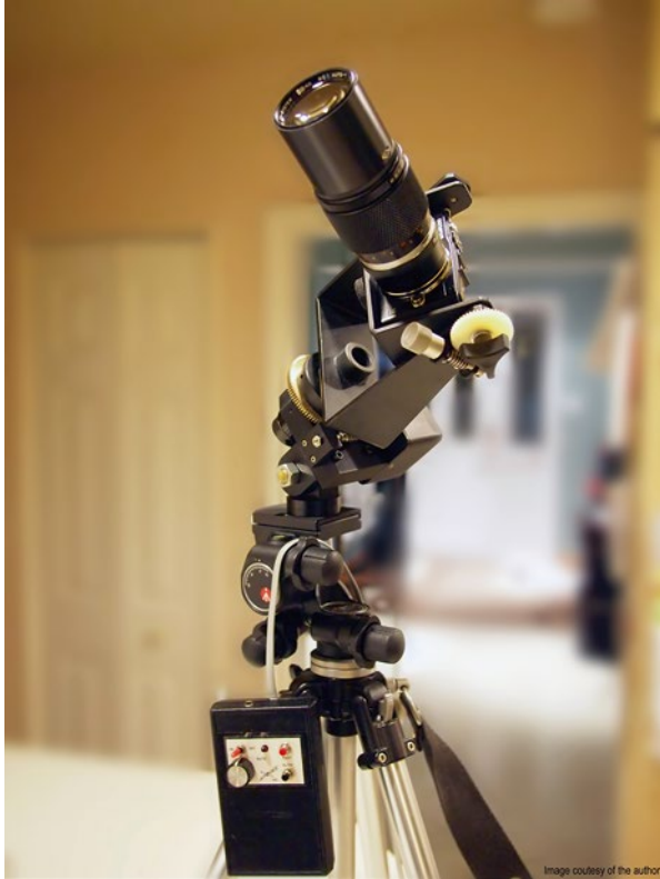
Fig. 1.4 Apogee MPFM on Manfrotto 410 geared tripod head and with OM series 200 mm f/4 lens. Both Olympus lens have retractable sun shades which double for dew shields at night
