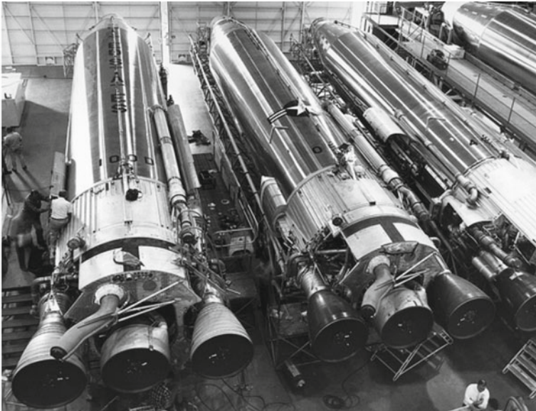
Atlas rockets under construction at the Convair/General Dynamics Kearny Mesa plant. (Photo: San Diego Air & Space Museum)
