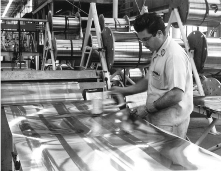
Cutting the thin metal skin for an Atlas rocket. (Photo: San Diego Air & Space Museum)
