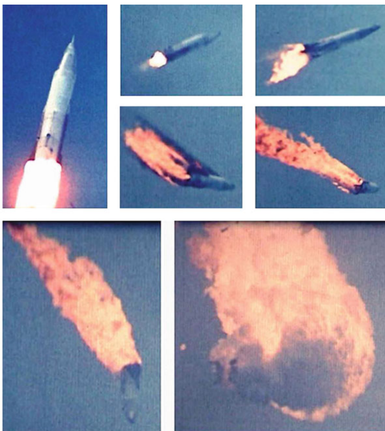
When Atlas 6A became erratic after lift-off it had to be destroyed by the range safety officer. (Photos: NASA)
