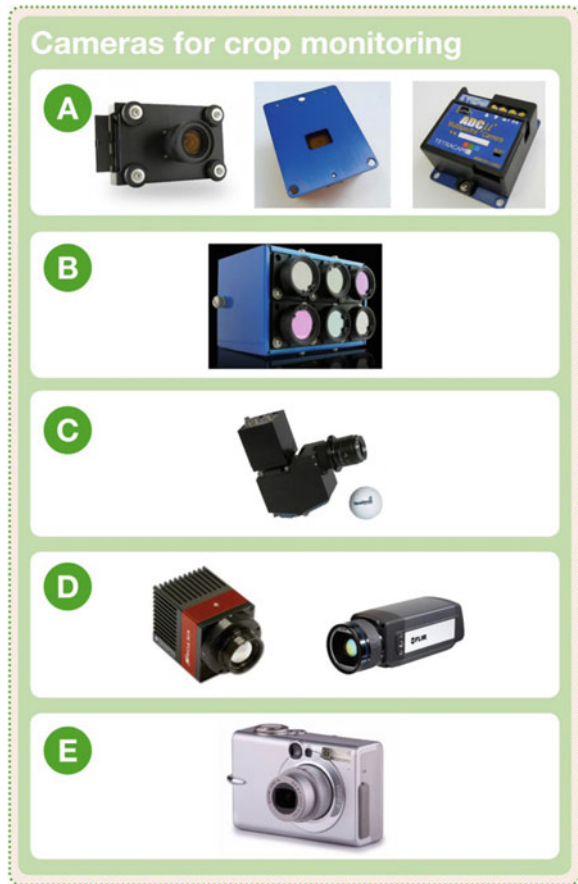
Fig. 1.3 Different categories of imaging systems for remote-sensing evaluation of vegetation. These include RGB/CIR a multispectral; b hyperspectral; c thermal; d conventional RGB; e cameras
