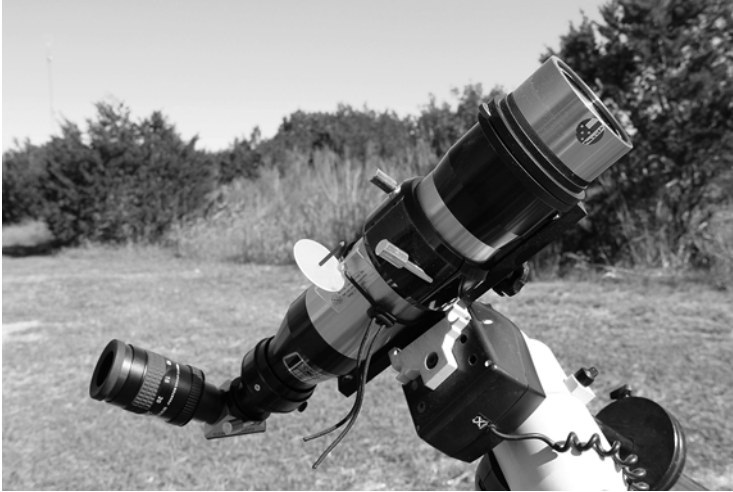
Fig. 1.1 Internally double-stacked Coronado Maxscope 60 mm, 400 mm focal length, Hydrogen-alpha dedicated solar telescope. (By Erika Rix)
