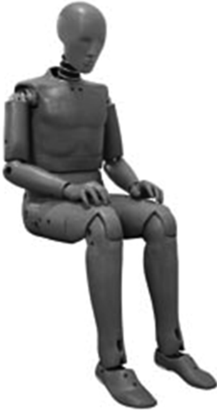
Fig. 1.3 Photograph of a Hybrid III dummy. (Courtesy of Humanetics Innovative Solutions, Inc.)
