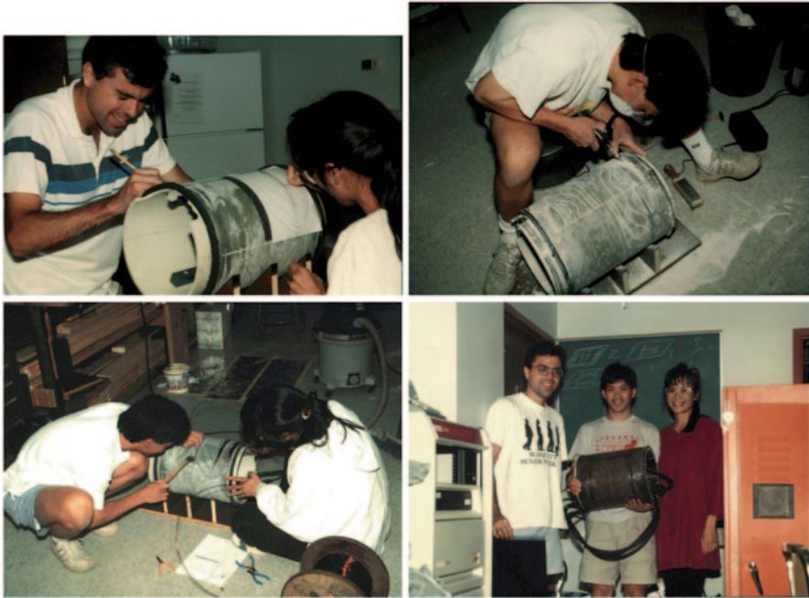
Fig. 2.1 Top left to bottom right : the sequence of making the gradient coil for performing EPI and first fMRI experiment. Eric, his wife Denise, and I made this in 36 h over the weekend before SMR. After designing the coil layout on his NeXT computer, Eric printed out the sheets, which we traced on to the PVC (i.e., sewer) pipe. These patterns were then gouged out with a Dremel tool (we went through several), and the wires were literally hammered in. Then, the next layer of epoxy was applied, and the process was repeated. SMR Society of Magnetic Resonance
