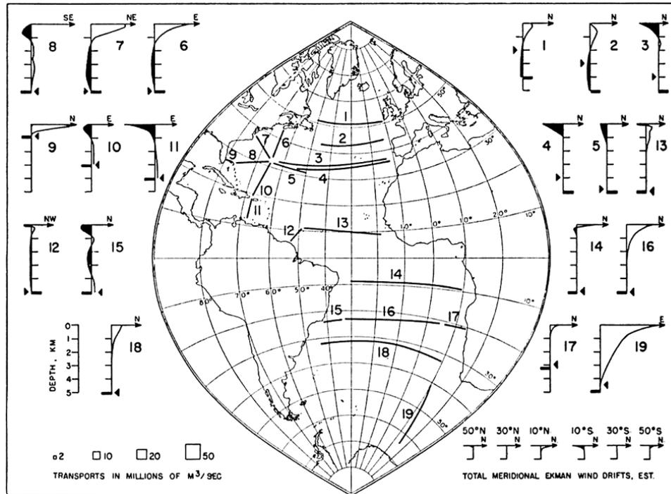
**Figure 5.** Geostrophic transport per unit depth across sections of the Atlantic Ocean, reproduced from *Stommel* (1958). The Ekman transports are shown in the lower right corner. For each section, the arrow points to the maximum depth of the data and the solid bar the bottom of the ocean.
