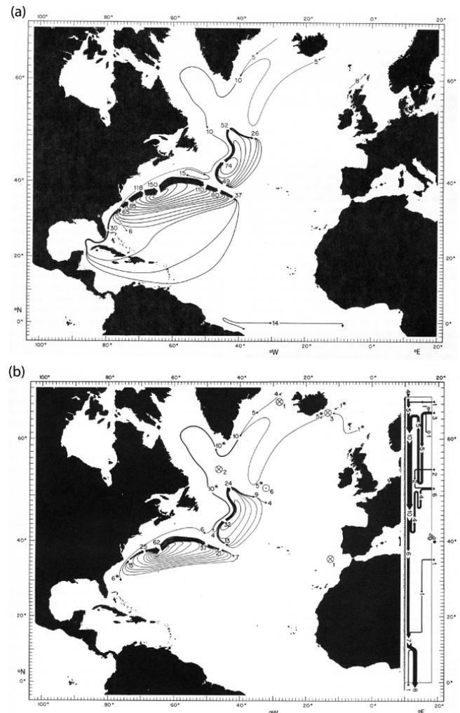
**Figure 3.** The North Atlantic circulation according to Worthington (1976) of the total water column (a) and the deep waters (colder than 4°C) only (b). Panel (a) does not show the 1 Sv of Mediterranean Water formation. The side insert of (b) is a meridional box model showing exchanges with layers above and across the equator, with 7 Sv net export to the southern Atlantic in this layer.
