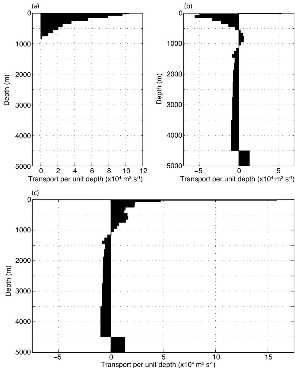
**Figure 6.** Meridional zonally integrated volume transport per unit depth at 24°N across the Florida Straits (a), the mid-ocean (b) and combined Florida Straits plus mid-ocean (c). Figure produced from Table 5 of *Hall and Bryden* (1982).
