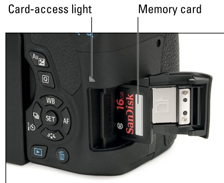
Figure 1-3: Insert the memory card with the label facing the back of the camera.
