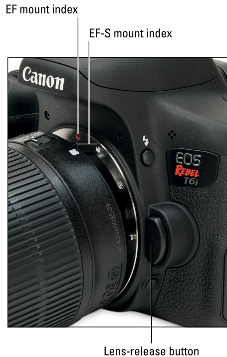
Figure 1-1: Align the mounting index on the lens with the one on the camera body.
