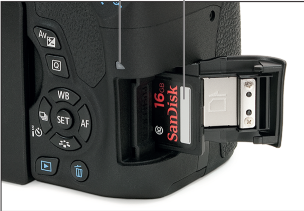
Figure 1-3: Insert the memory card with the label facing the back of the camera.
