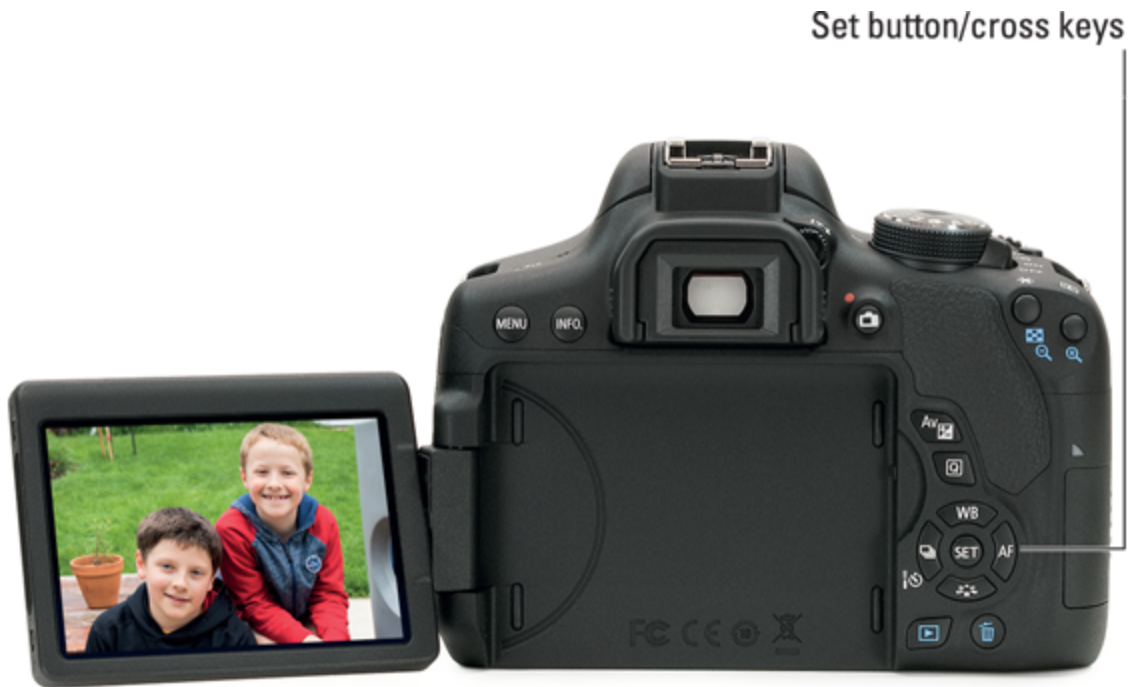
Figure 1-5: You also can rotate the monitor away from the camera to find just the right viewing angle.
