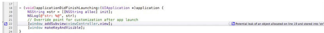
Figure 2–6. Static Analyzer reports a potential leak of an object allocation on line 19 and stored in str.
