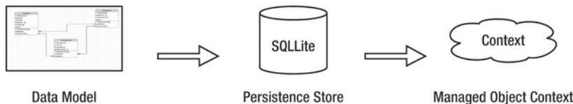
Figure 1–8. Core Data initialization sequence
