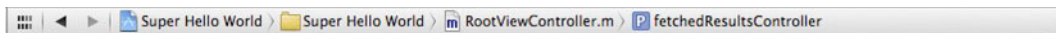
Figure 2-7. The Jump Bar is a navigation tool that is always available to the editor it is above. It is also available in Instruments to perform the same types of tasks.
