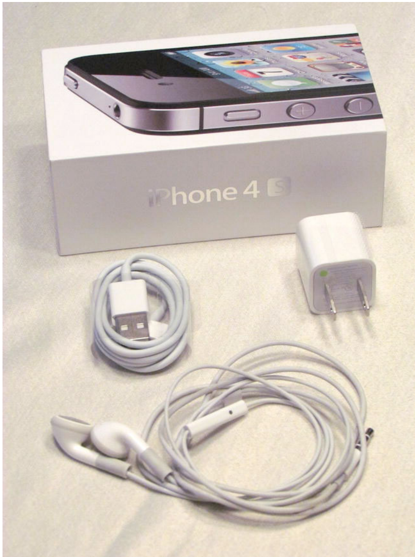
Figure 1–2. The content of that nice iPhone box usually consists of a USB-to-dock connector cable (left), a USB power adapter (right), and a stereo headset (bottom). You can find your complimentary Apple sticker in a packet inside the box.
