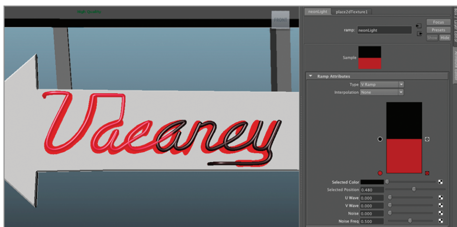
Figure 1.7 Move the black color of the ramp up and down; the color updates on the tube geometry in Perspective view.
