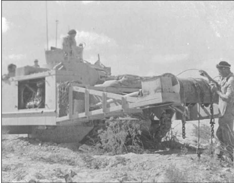
A useful view of a Matilda Scorpion I preparing for action. The commander is in his cupola, one crew member is checking the joints on the wire and chain flails, while the flail operator is in his engine box on the side.
