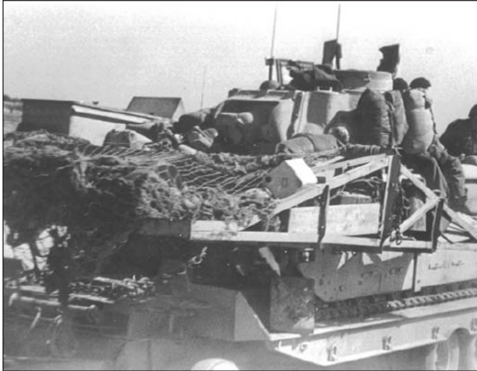
A Matilda Scorpion II heading west on a transporter. The flail apparatus is camouflaged, but the nearside arm can be seen, along with the engine box on the far side.
