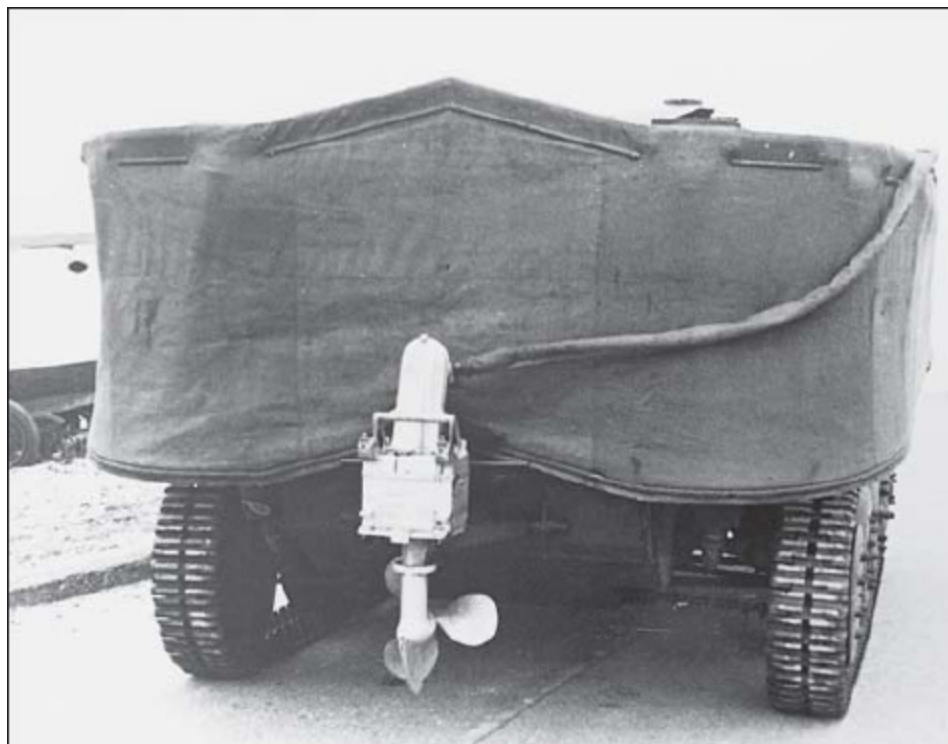
The prototype Tetrarch DD prior to its first swim in Langstone Harbour. The marine drive equipment can be seen at the back; notice how the propeller, which is controlled by the line that vanishes over the screen on the right, faces forwards.
