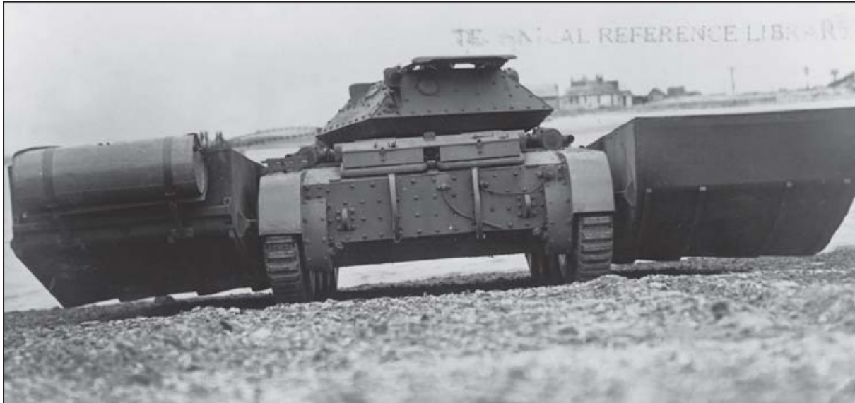
Another Covenanter, here fitted with a pair of floats, prepares to take the plunge into Fareham Harbour. Notice how the long-range fuel tank, normally carried at the back of the Covenanter, has been transferred to the port-side float.
