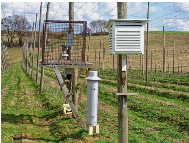
Figure 9: Spore traps in a hop yard for determining the number of zoosporangia; pictured in the foreground is the weather station
