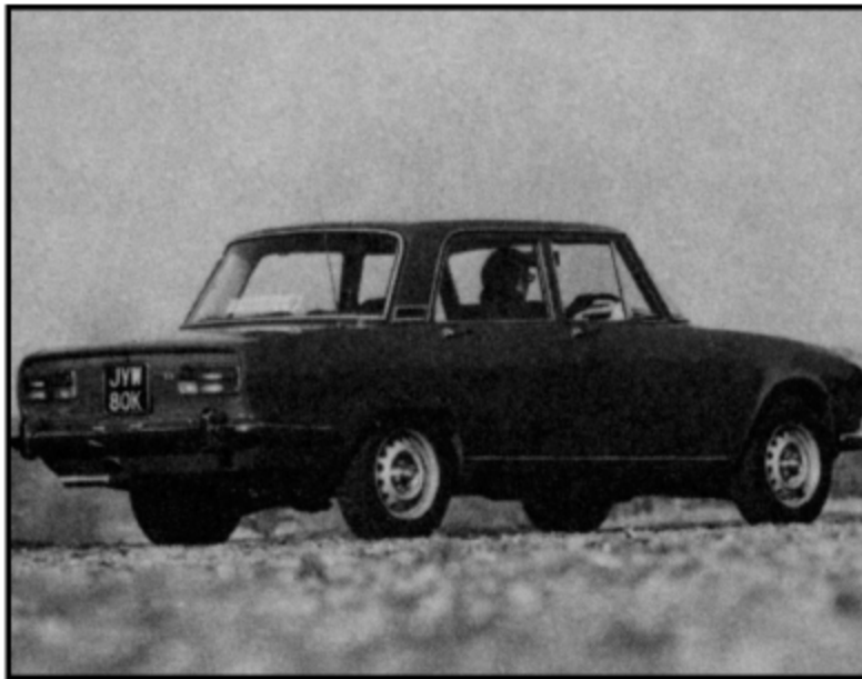
The rear of the 2000 Berlina, with the lamps slightly recessed in the tail panel
