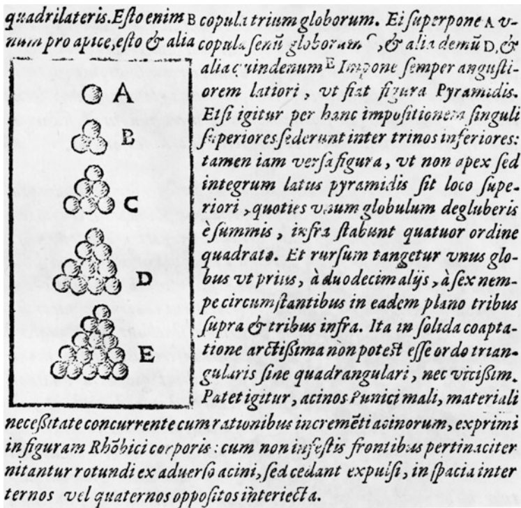
Fig. 2 Kepler's description of the FCC "cannonball" packing. [Image courtesy of the Division of Rare and Manuscript Collections, Cornell University Libraries.]
