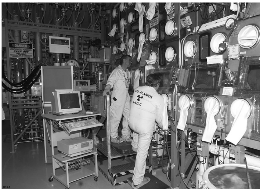
Fig. 1.2 A modern laboratory with a bank of gloved boxes for carrying out experimental chemistry of transuranium elements. (Reproduced by permission of Los Alamos National Laboratory.)
